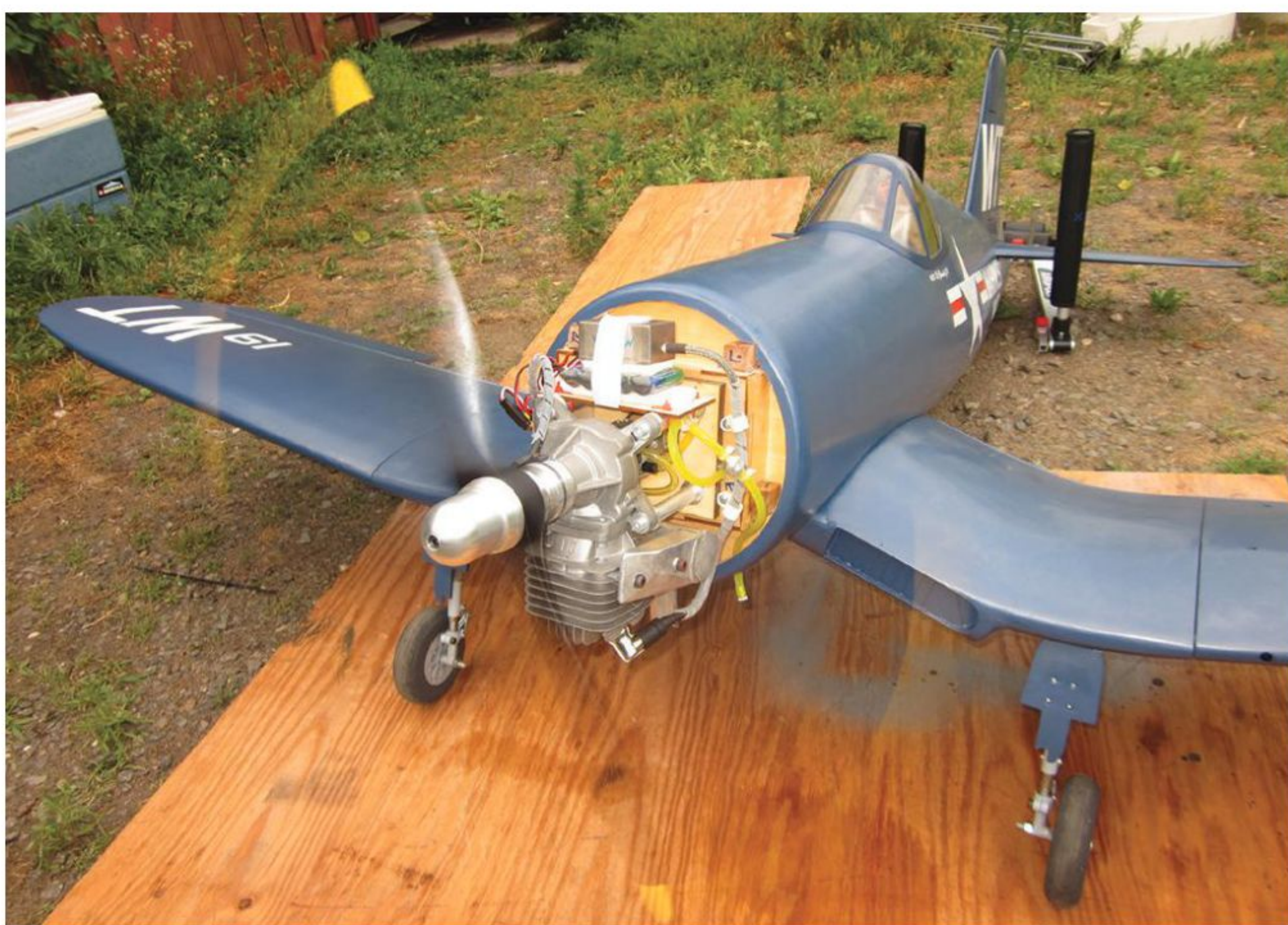
Placing a large sheet of plywood under your warbird while test running the engine will keep flying dust and debris to a minimum.
