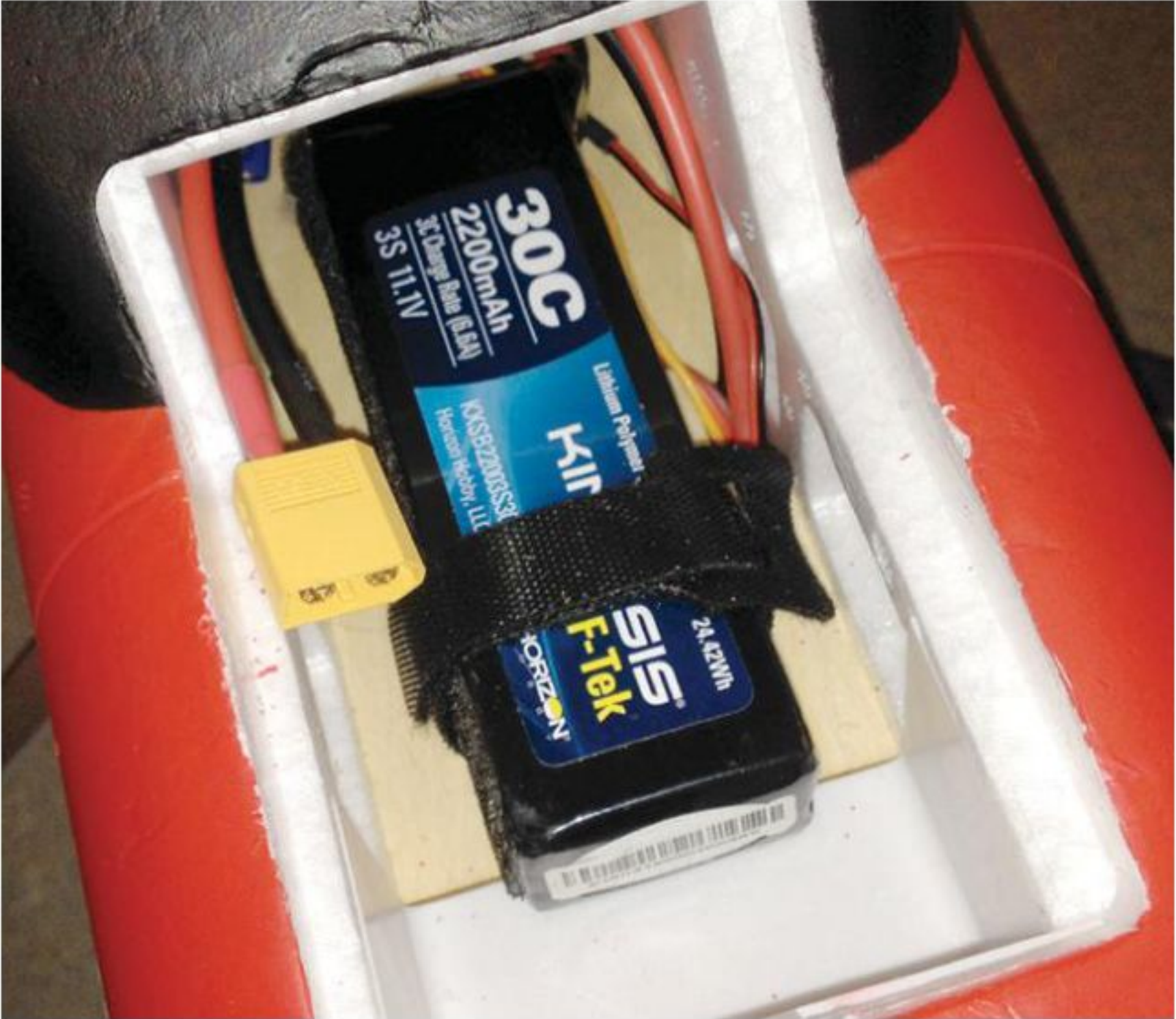
There's plenty of room for any battery pack. I used a Kinexsis 2200mAh LiPo pack with an adaptor to match the speed control's XT60 connector plug.
