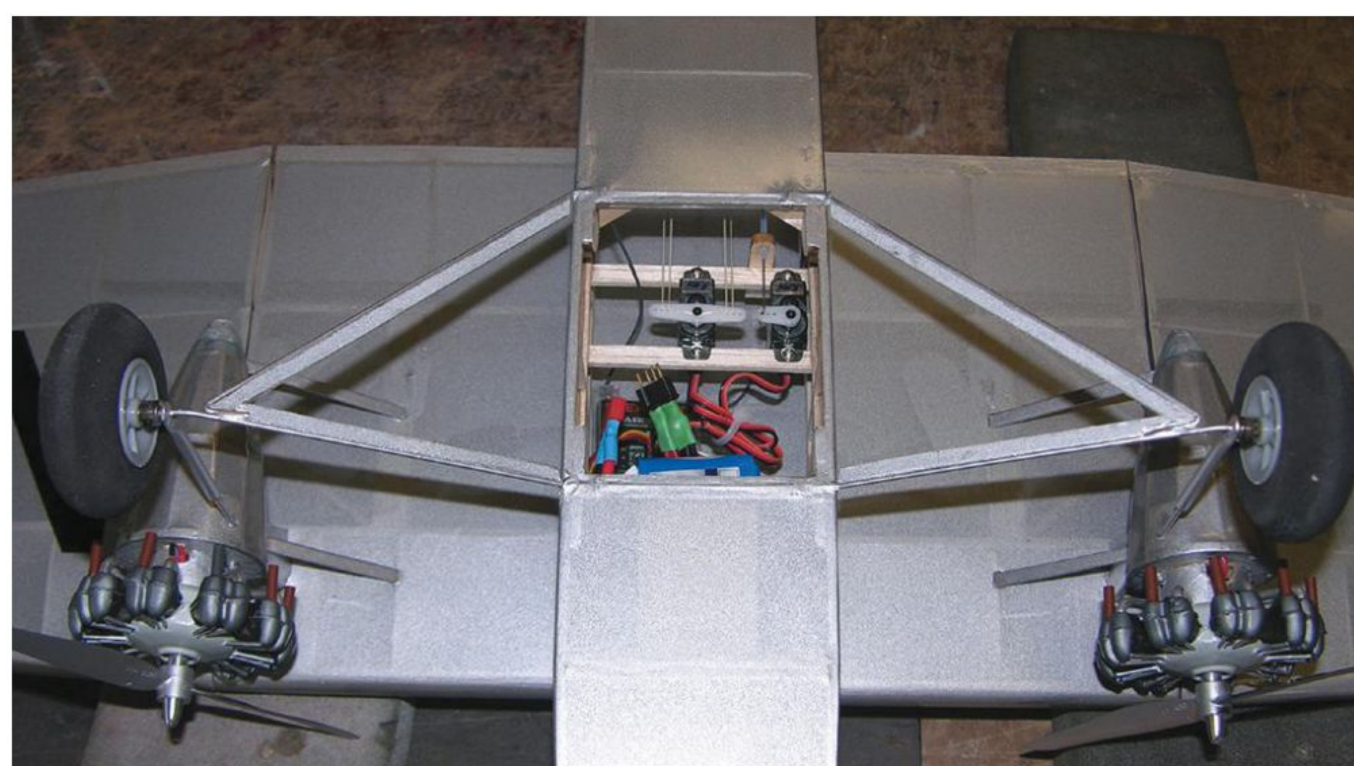
The rudder and elevator servos are accessed through the battery hatch on the bottom of the fuselage. The battery is mounted on the tray with Velcro at the front of the opening.
