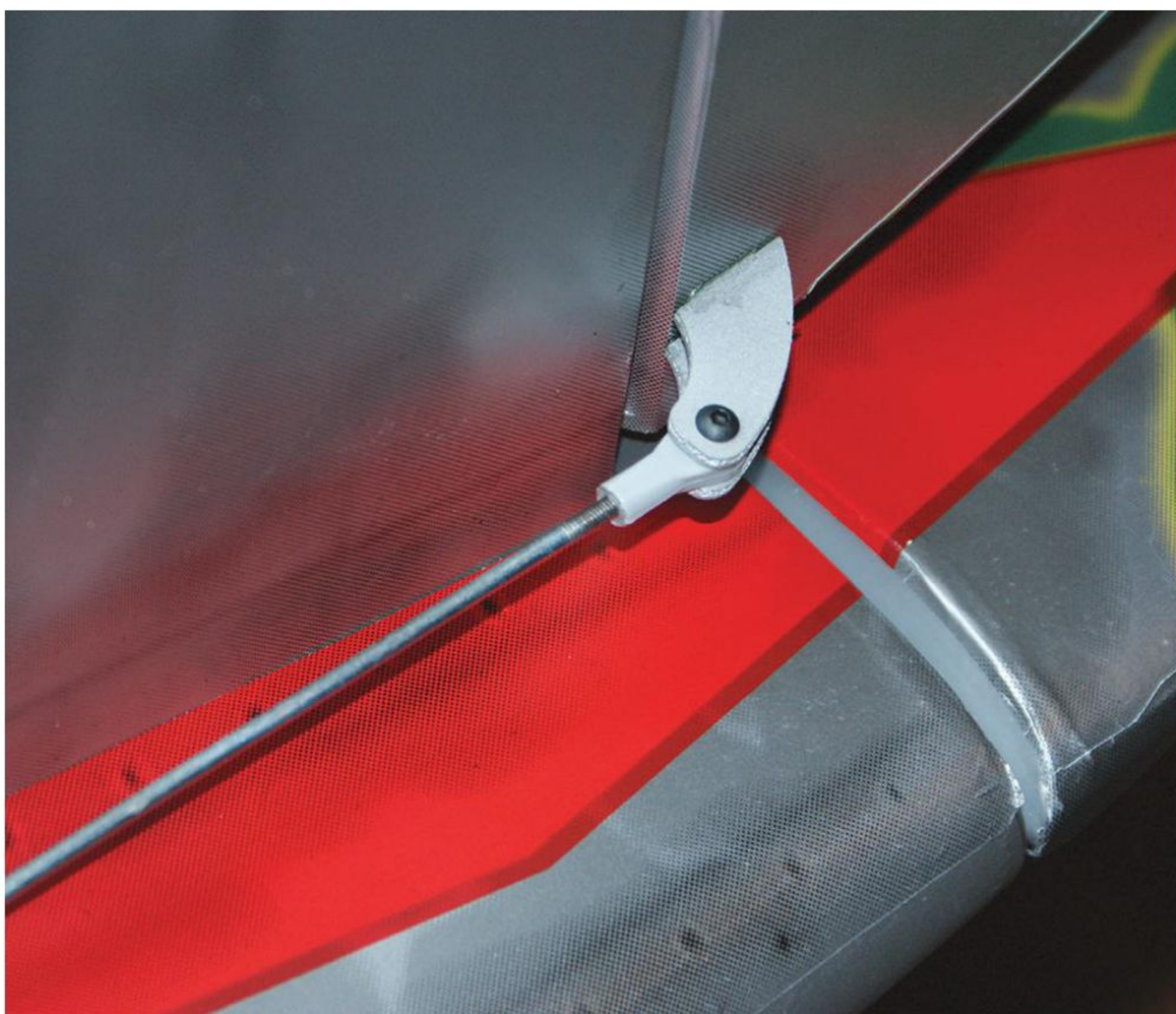
A slop-free control system is provided that uses heavy duty rods, ball links, and G10 fiberglass double-arm control horns. The control horns are painted silver to match the covering.
