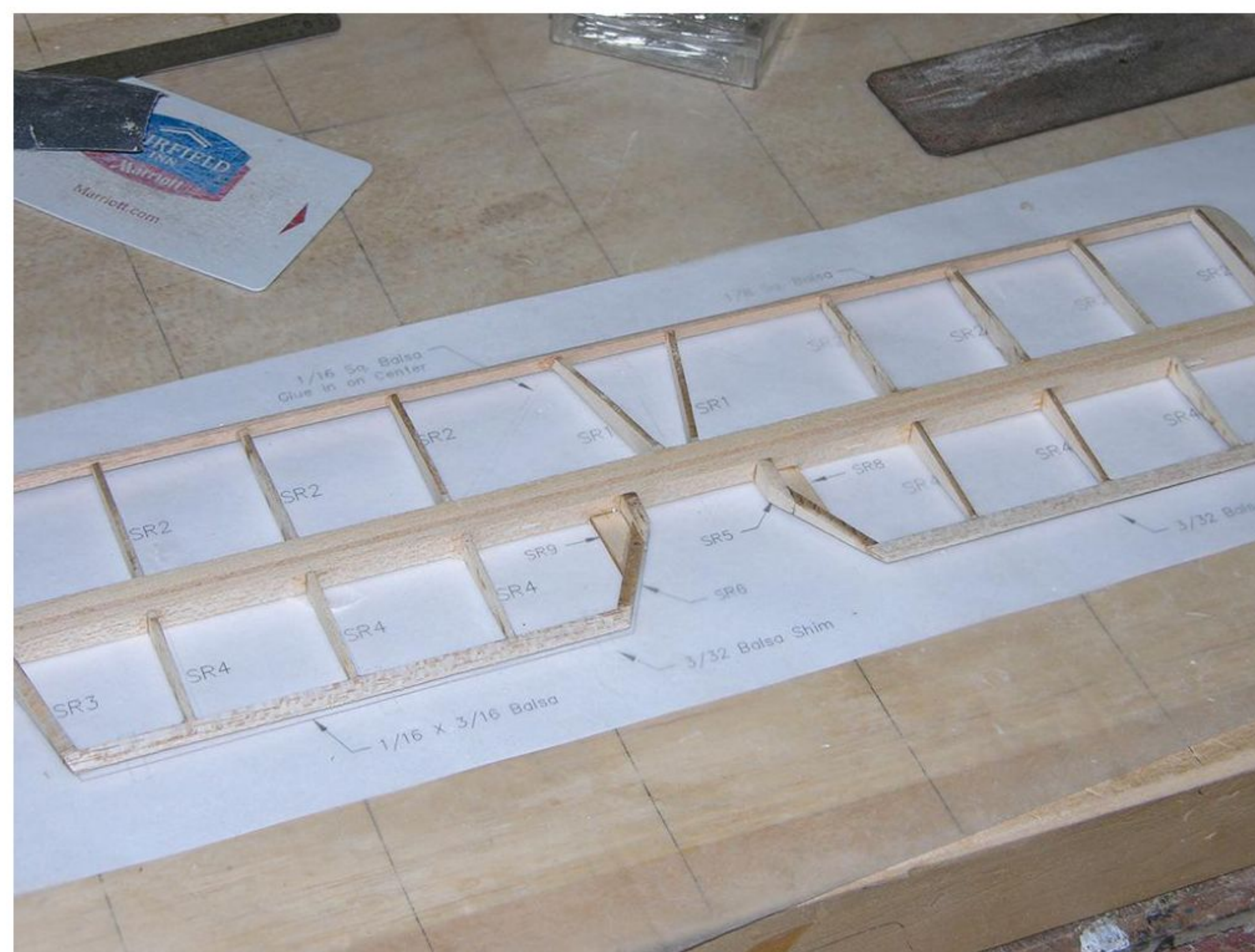
The horizontal stabilizer/elevators are framed directly over the plans.
