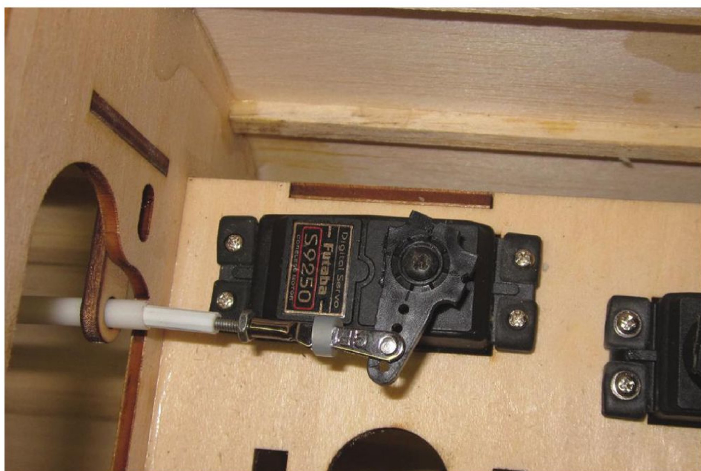
Take your time and set up the throttle servo and linkage so you get the full range of travel from full off to full throttle.
