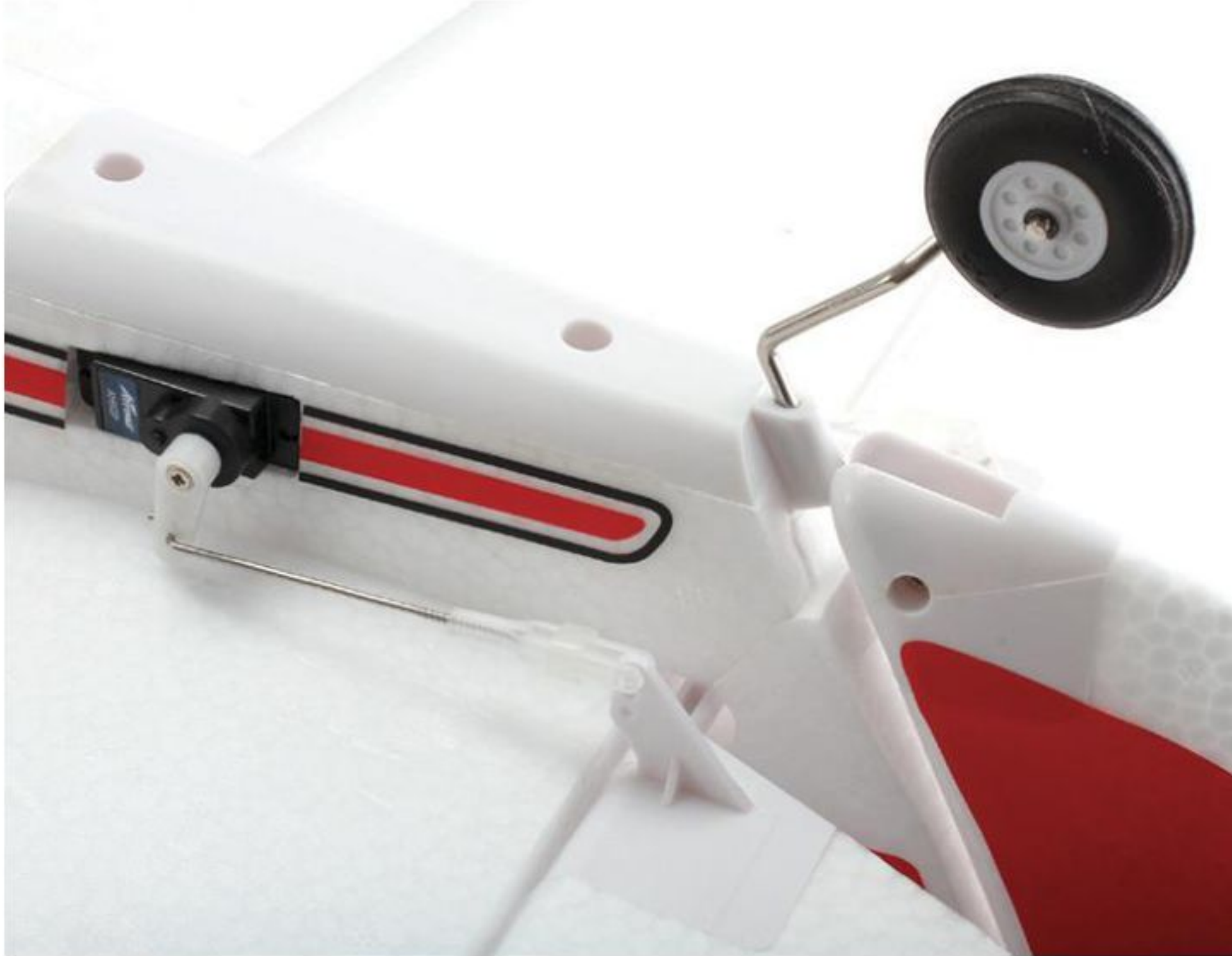
The rudder and elevator servos are located in the tail.
