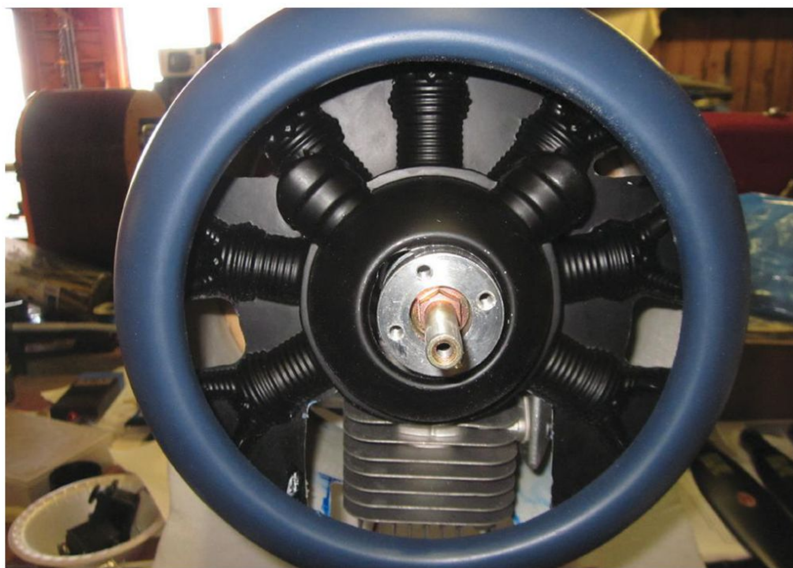
Securely install your engine cowl and trim the air inlet and exit openings to maximize cooling airflow around and through the engine cylinder fins. Be sure to test run your engine with the cowling installed before your test flight.
