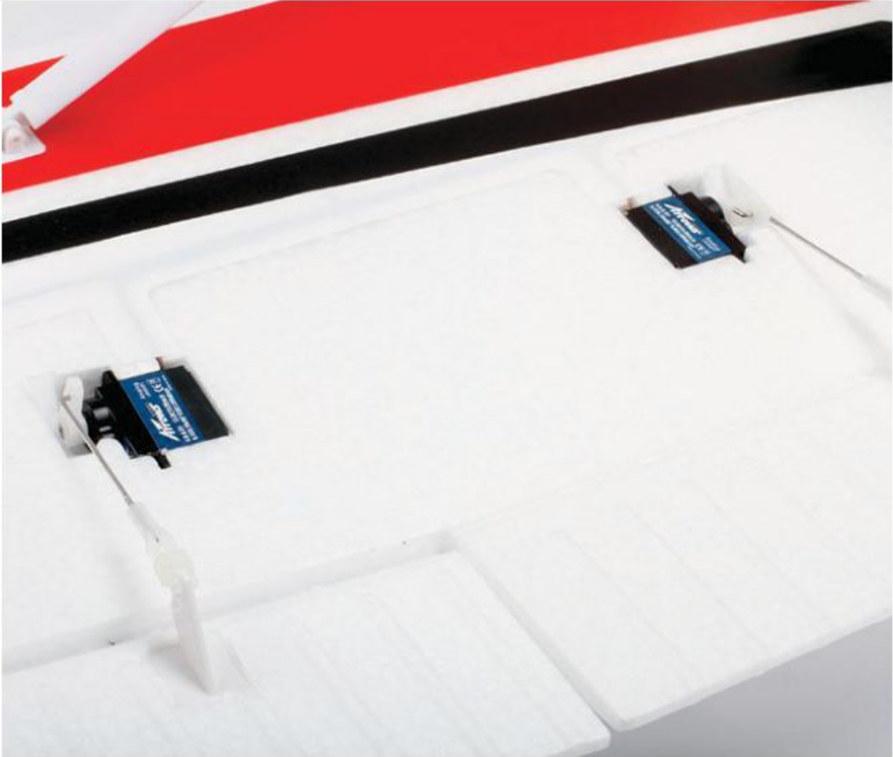
Both the aileron and flap servos come installed in the wing with the linkage attached.
