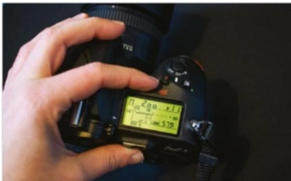
**2 Select settings** Put your camera in Manual mode. Set the shutter speed to 1/200sec and ISO to 100. We're going to start with our aperture at f/11, but we can adjust this with the flash power if need be.
