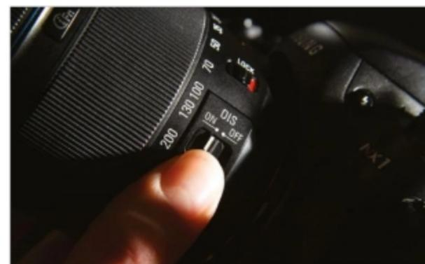
**3 Activate stabilisers** Turn on image stabilisation, whether this is built into the camera or the lens. If a 'Hybrid IS' mode is available, use this, as it's better for handheld shooting, covering rotational movements.
