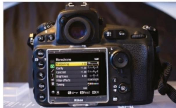
**3 Change to monochrome** For an easy B&W conversion, apply a monochrome picture style setting to your file in-camera. Note it will only be applied to a JPEG – a RAW file will need to be converted in editing software.
