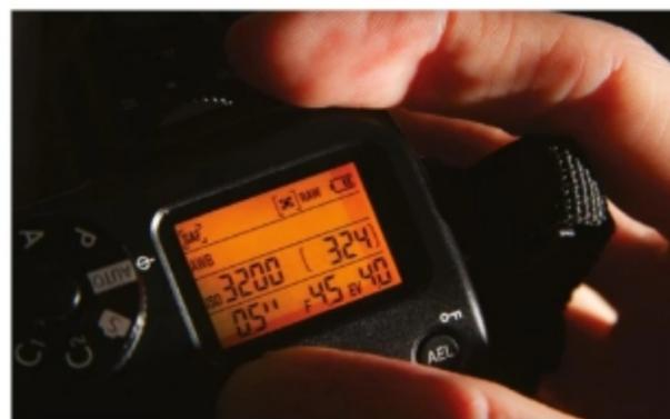
**5 Set exposure** Find out the stabilisation ability of your kit, and set the shutter speed at the EV value below the minimum unsteadied handholdable speed. For a 60mm lens (1/60sec) 5 stops slower would be 1/2sec.
