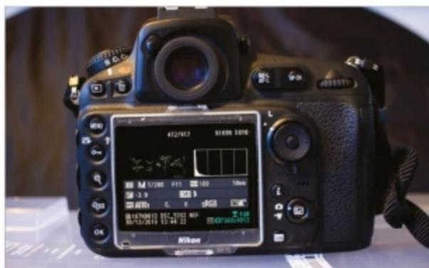
**5 Take a test shot** Take a shot to test the flash strength, direction and camera settings, and tweak if necessary. Don't fully rely on your LCD screen – use the histogram as well to read what is happening in the image.
