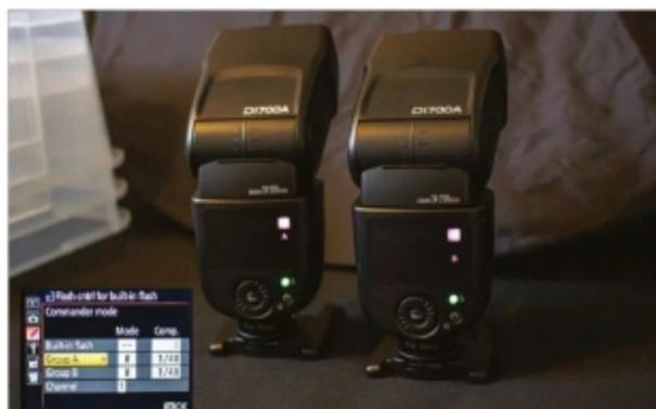
**4 Position lights** Place two flashguns behind and below the subject so that the flashes are pointing up. Our flashes are firing at the same strength (1/40) in Manual mode, which we can control independently from our camera.
