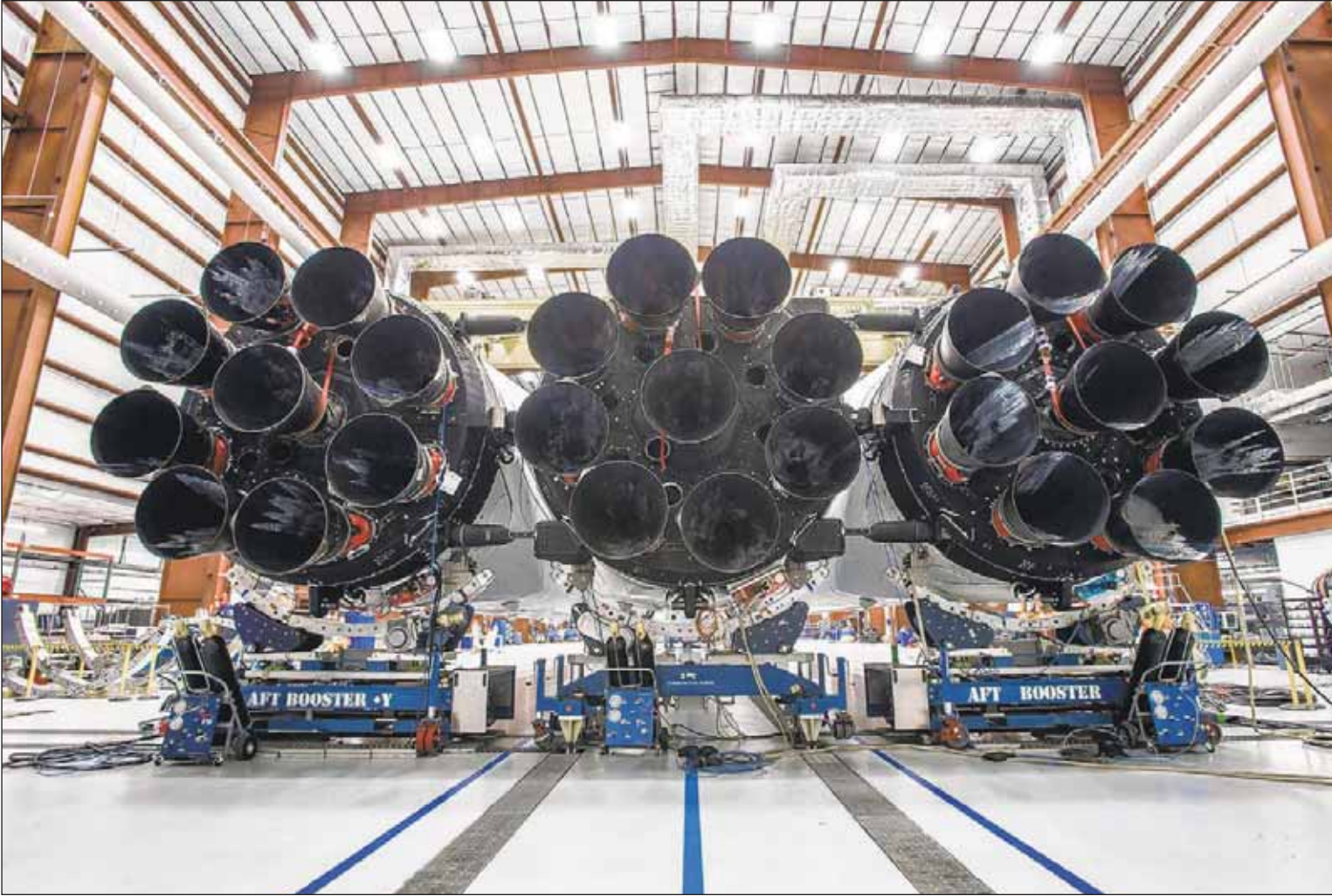
SPACEX'S Falcon Heavy rockets have 27 engines that create a thrust equal to 18 Boeing 747 jetliners. They also create pollution.
