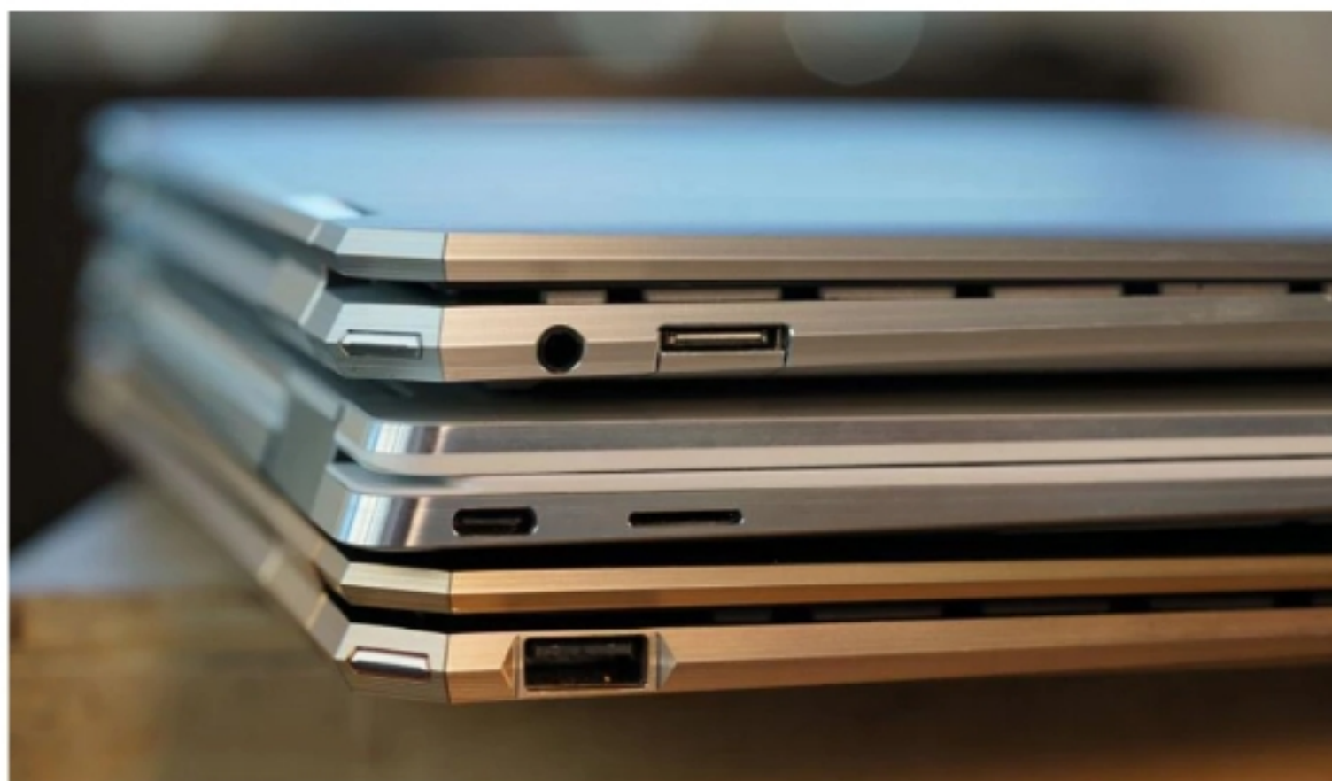
The newest HP Spectre x360 13t (top) features a USB Type-A port using a drop-down latch. The Dell XPS 13 2-in-1 7390 (middle), throws USB Type A under the bus. On the bottom is an older Spectre x 360 13t with the fully exposed USB Type-A port.
