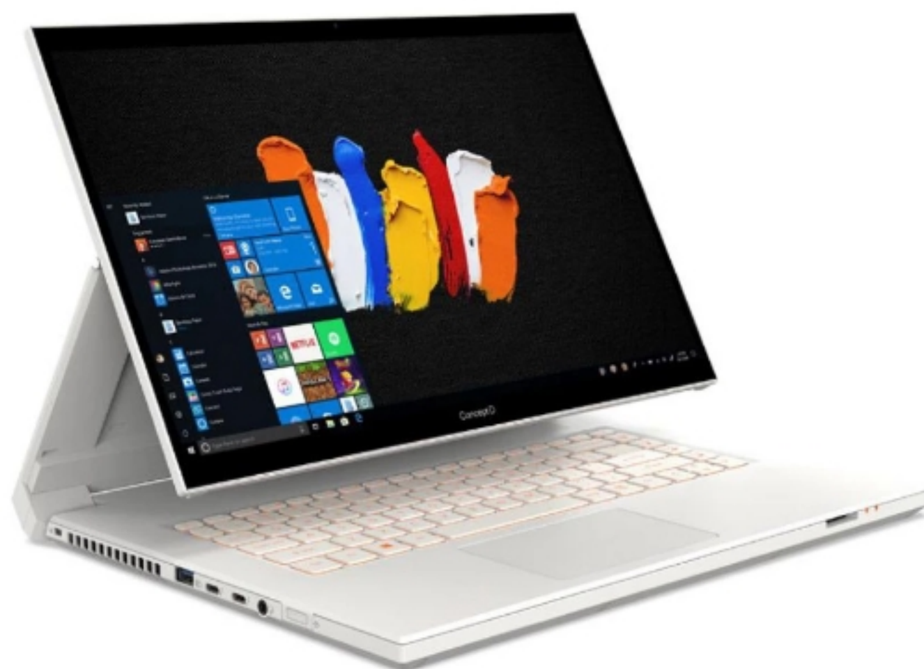
The Acer ConceptD 7 Ezel's display has two hinges, one at the bottom and one at the middle, so it can work as a clamshell or "float" at a number of angles for viewing or drawing.
