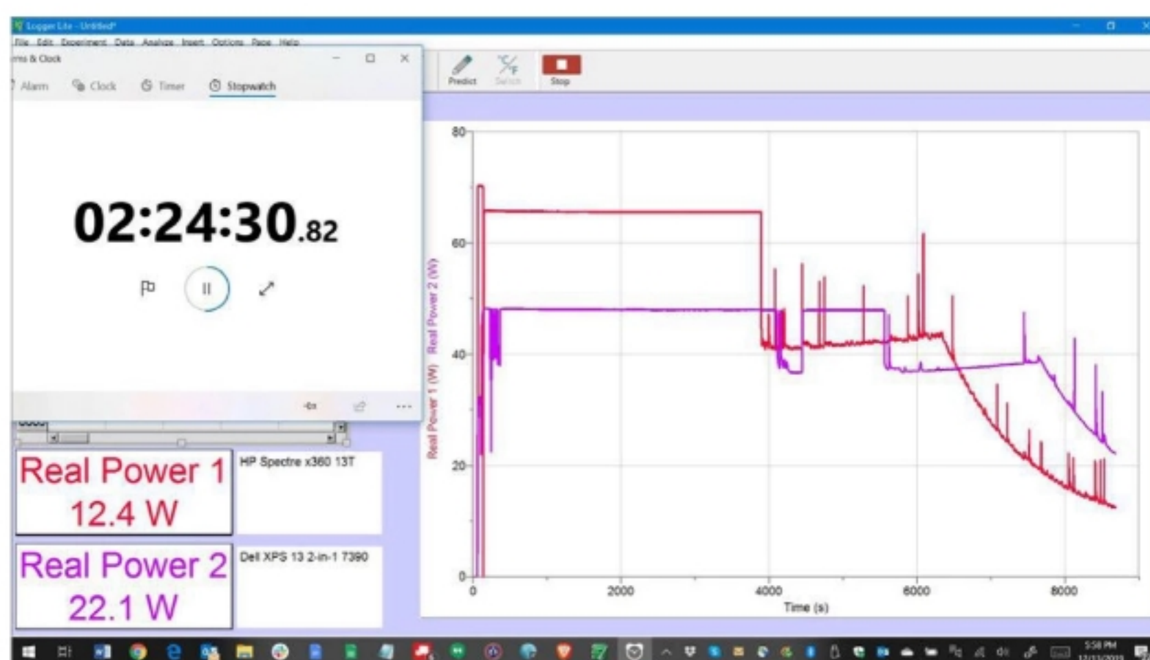
The HP's larger 65-watt power brick let it run and charge faster than the Dell's 45-watt brick. Beyond about 20 percent though, the Dell's performance lead comes back, and it charges to 93 percent in about 2.5 hours.
