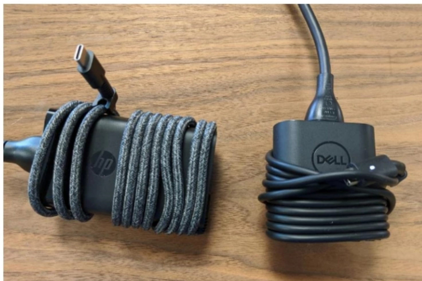
The HP's (left) power brick is 65 watts and features braided cabling. The Dell's (right) is smaller and puts out only 45 watts. It does have a cool LED indicator top to let you know it's actually plugged in.
