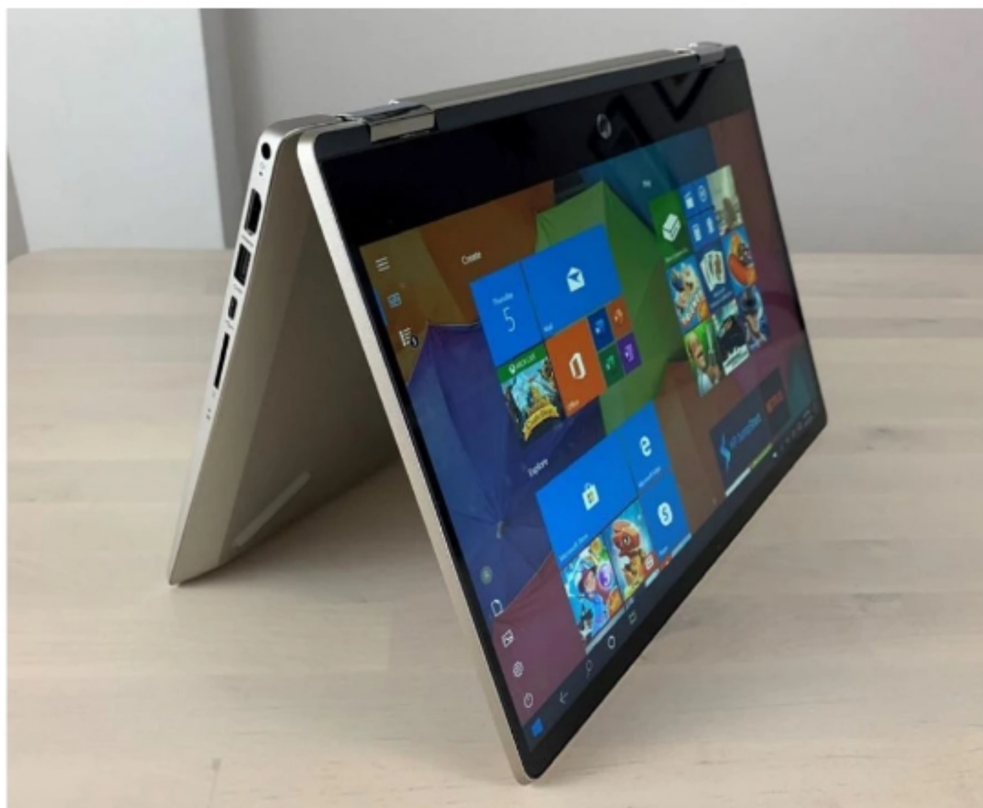
As a 2-in-1 laptop, the HP Pavilion x360's lid can bend all the way around, perfect for tablet use or for tenting on a desktop.
