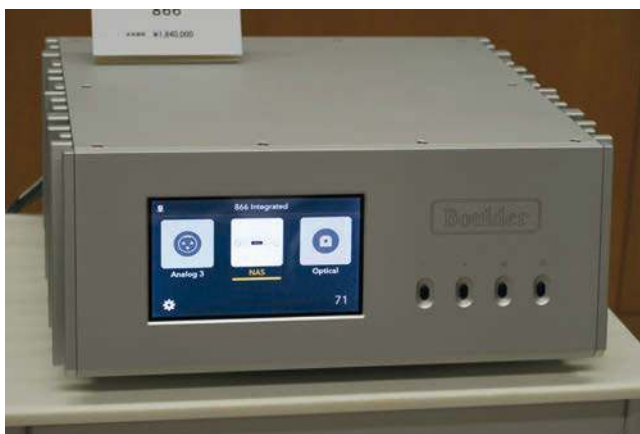
Boulder's unusually styled Model 866 caught quite a few peoples' eyes. The 200W integrated amplifier features a full-colour touch screen display. This is used to show the available inputs – you can even have pictures of your own sources, or show the unit status and it is also used during the unit set-up procedure. Price 1,840,000¥.
