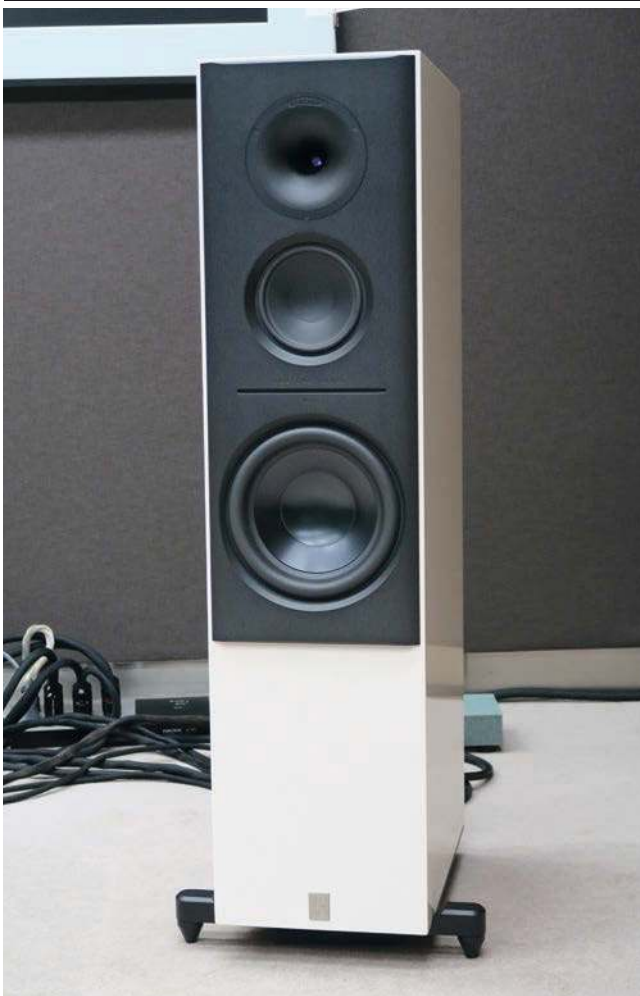
Lansche Audio from Germany showed its new 5.1 loudspeaker. This features an improved version of their plasma driver. This driver covers the range from 2,500Hz to 150,000Hz and gives the 5.1 phenomenal speed and transparency. Driven by Mola Mola electronics and an EMM Labs TX-2 SACD transport, the 5.1s produced what was said by many to be the best sound in the show. Price 4,950,000¥ per pair.
