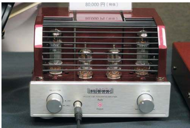
Just to show that not everything at the show was priced at stratospheric levels, Triode showed its Ruby stereo integrated amplifier which will only set you back 80,000¥. This uses one EL84 tube per channel delivering 3W into 8 ohms. Combine this with a pair of headphones and a good quality streamer and you have the basis of a compact, good sounding audio system that won't break the bank.
