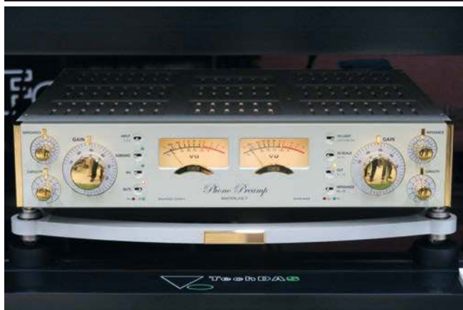
The Masterline 7 phono stage from Swiss professional audio products maker HSE Swiss Audio Lab gets the prize for the product with the most stunning looks in the show. Components that are matched to within 0.2%, a cabinet with 20 mm thick walls, that is milled from a solid block of aluminium, silver-Teflon wiring and a design life of 30 years go some way to explain the eye-watering 8,700,000¥ price.
