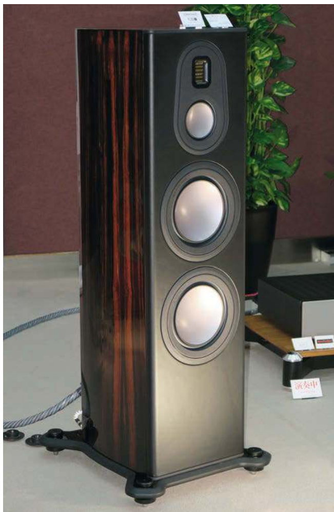
Monitor Audio's PL 300 II. This three-way design features an interesting ribbon type tweeter. This has what the maker describes as a Micro Pleated Diaphragm and was custom designed for this model. Overall this loudspeaker is nicely put together. Priced at a very reasonable 1,600,000¥ per pair.
