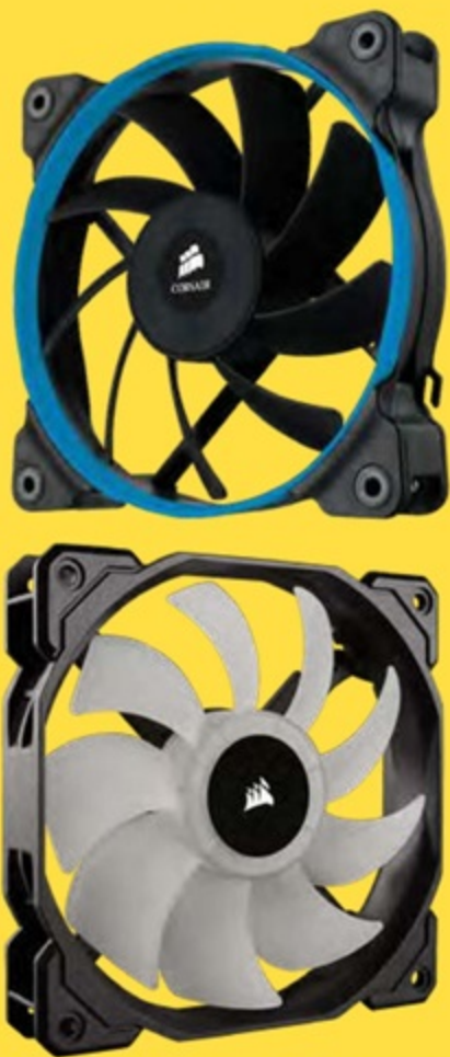
High-airflow fans have narrower blades with larger gaps between whereas high static pressure fans have large, more angled and closely spaced blades
