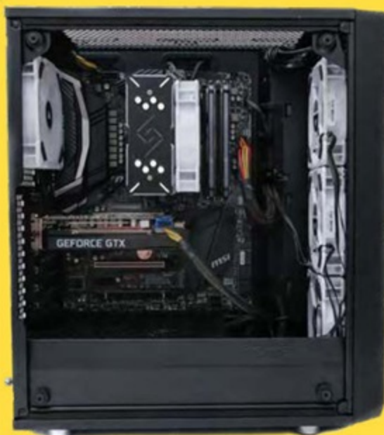
Many fans in the front of a case produces a positive pressure environment. Many fans exhausting air out the back creates a negative pressure environment
