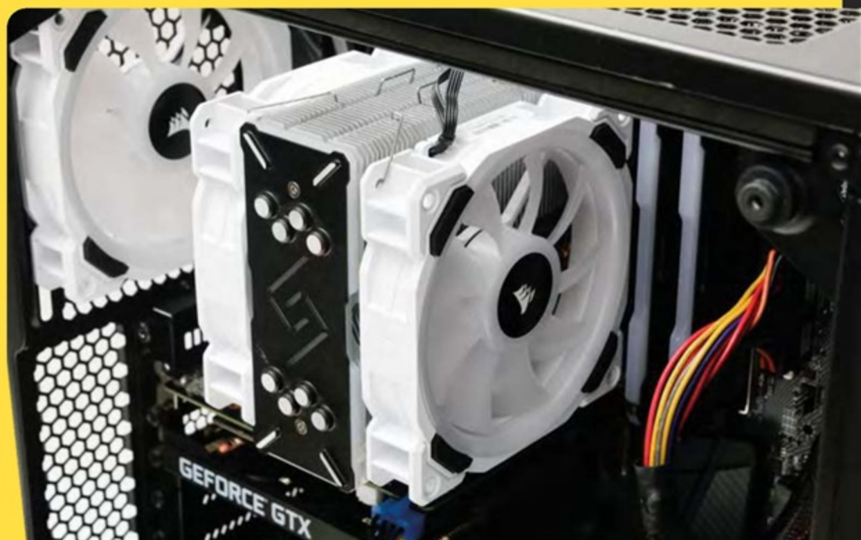
Adding a second fan to the CPU cooler does more than most other fan configuration changes
